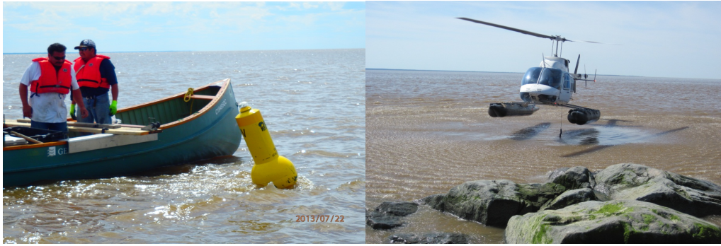
Photos 1 and 2: Surface buoy marking a mooring station (left), Locating the saltwater front near the shore by helicopter (right)
